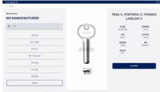
1.- Screen for entering model empty. 2.- Screen for entering model with suggestions and model TE-T60 selected (with information showing an image, manufacturers that use that key and equivalent references of other manufacturers)
